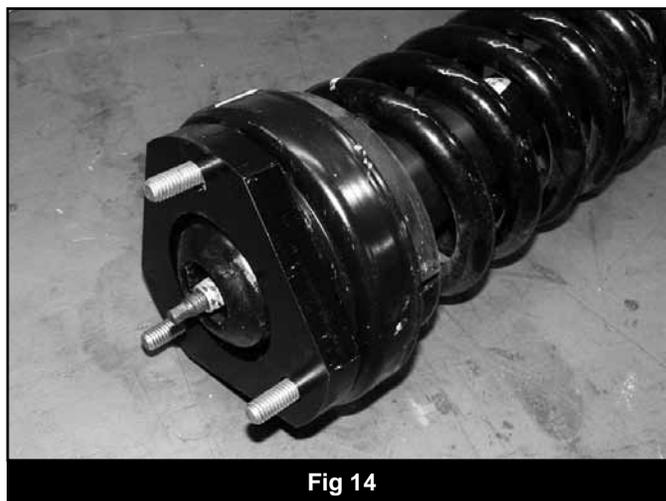
23. Install the modified strut assembly in the vehicle as it was removed. Fasten the upper strut mount to the frame with 7/16" nuts, lock washers and flat washers. Torque nuts to 40 ft-lbs.
