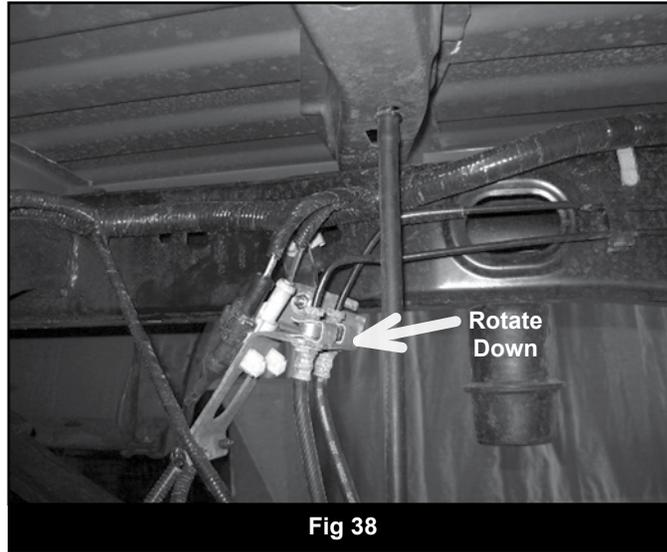
22. Attach the brake line to the relocation bracket with a ¼" nut and ¼" USS washer (BP #774). It may be necessary to rotate the OE brakeline clip bracket to have the lines face 'down' for adequate slack. Torque to 15 ft-lbs.
