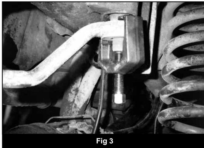
10. Disconnect the front anti-sway bar if present and save fasteners to reattach later.
