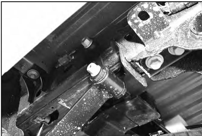
6. Grease and install the longer sleeve (166) in the frame end. Grease and install the shorter sleeve (165) in the leaf spring.
