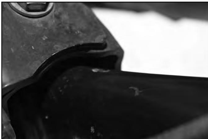
7. Adjust the arms to the desired length. Lengthening the arms will increase caster. Suggested length for 4-1/2" of lift is 24-9/16".
